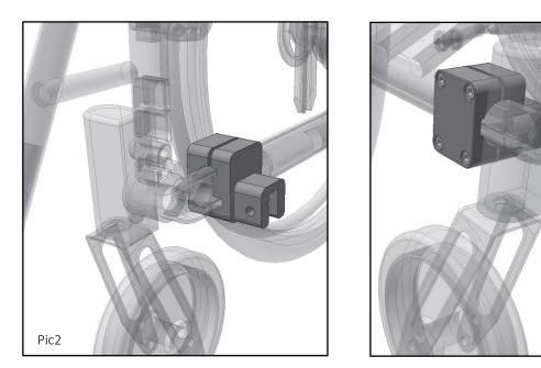
Mount the adapterbar (A) using the QR Pin (D) (Pic4).
