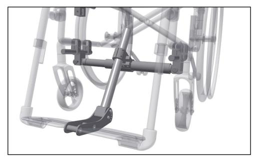
Mount the level tool onto the adapter bar fork (B). Remove the rear screws (E) in the fork that locks the rotation and make sure that the front screws (F) are a little bit loose so that the fork can be rotated. Check that the adapter bar fork (B) sits in the center of the wheelchair.
