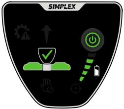
The calibration continues to be updated in background. For every update, the indication *calibration* blinks. Depending on temperature changes, etc., the calibration may need to be repeated. If this happens during use, stop, release the handle, and wait until the indication *calibration* to blinks.
