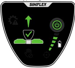
Only horizontal forces affect Simplex. Do not lift or push the handle downwards. Do not start steering before E-Drive is started. Simplex does not start if the force on the handle is too high. Then the indication release the handle is shown:
