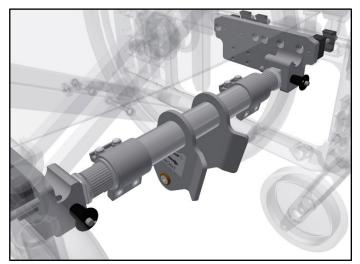
Now tighten all the screws (I) that holds the adapter plate in place.
