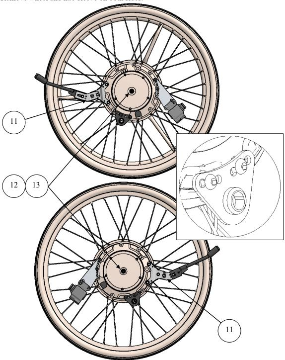
2. Check the correct placement for the eMove, and that it is axle Ø12,0 x 51 with part number: XOE-2530-B0 and Spacer with part number: XOE-25883-00.
