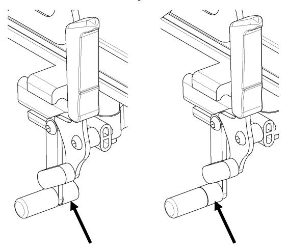
5. Move the spacer to the outside and adjust parking brake.
