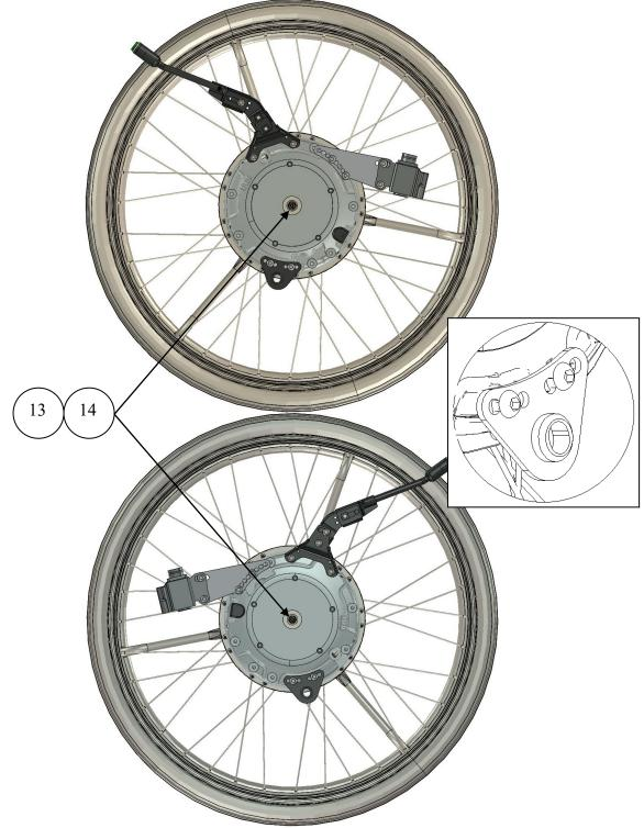
2. Check the correct placement for the eMove, and that the spacer with Part Number: XOE-25383-00 and axle Ø12 x 51 with Part Number: XOE-2530E-B0 is mounted.
