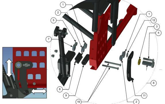
3. Assembly the plate and anti-tip devices (right side) according to picture. Different placement for the bracket is possible.
